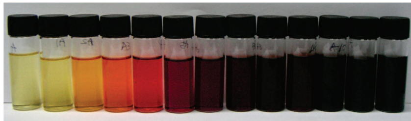
Figure 1. Photographs of the samples of 0.2 mmol of CuAc, 0.2 mmol of In(Ac) 3 , and 0.5 mL of dodecanethiol in 5 mL of ODE after heating at 240 °C for (from left to right) 1, 3, 6, 10, 15, 20, 30, 60, 120, 180, 240, 300, and 360 min.
